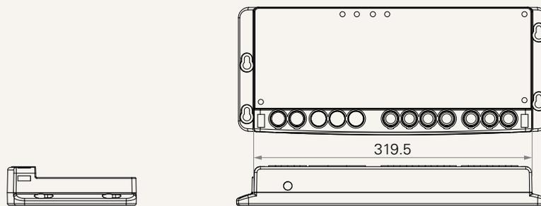
TP4 (power supply) and TBB (back-up power)
