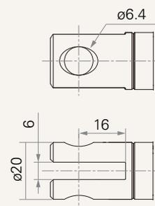
5 = Aluminum, U clevis, slot 6.0, depth 16.0, hole 8.0
