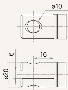
4 = Aluminum, U clevis, slot 6.0, depth 16.0, hole 6.4
