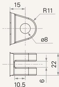
6 = Aluminum, U clevis, slot 6.0, width 10.5, hole 10.1, one piece casting with gearbox
